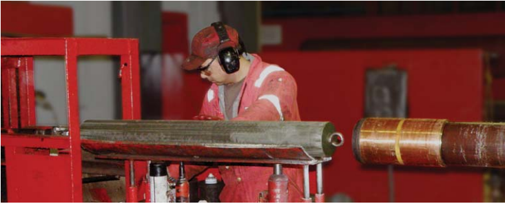
Figure 11.17 Drifting tubing before shipment to the wellsite.
