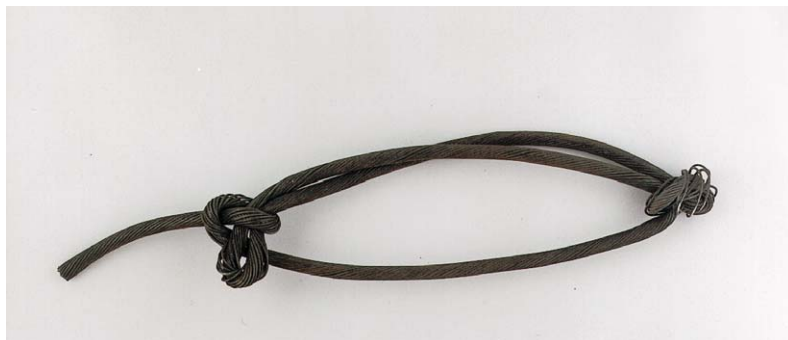
Figure 2.46 Knot in wireline caused by excessive underbalance.
