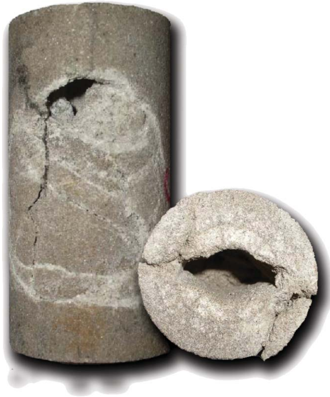
Figure 3.4 Failed TWC samples (photograph courtesy of Boris Tarasov, University of Western Australia).
