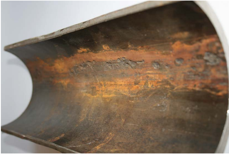
Figure 8.6 Corroded 13Cr tubing.
