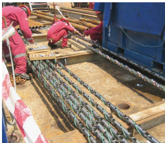
Figure 2.54 Loading shaped charges (photograph courtesy D. Thomas).
