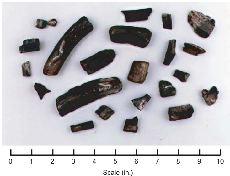
Figure 11.1 Debris from the milling of a packer.
