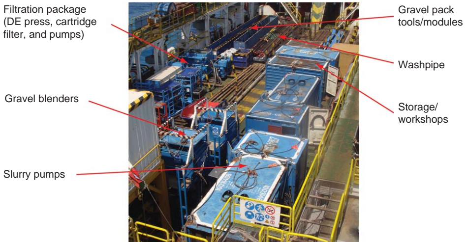
Figure 11.19 Completion equipment and services on a barge (photograph courtesy of Dave Clark).
