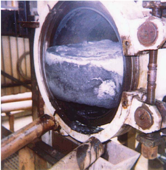
Figure 7.24 Hydrates in a pig receiver.
