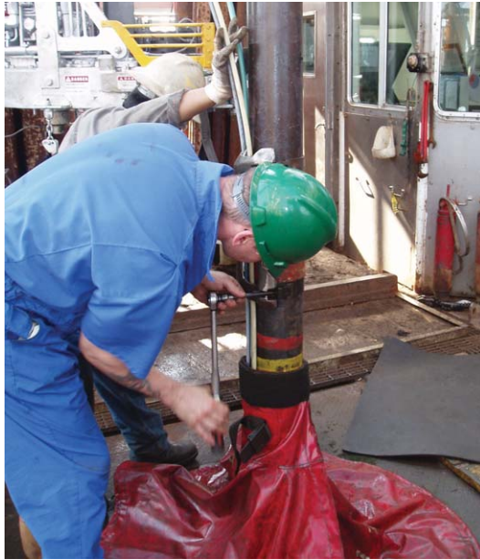
Figure 11.26 Tightening a cable clamp using a torque wrench (photograph courtesy of Danny Thomas).
