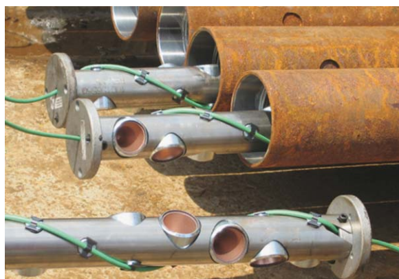
Figure 2.55 Loading guns into the carrier (photograph courtesy D. Thomas).
