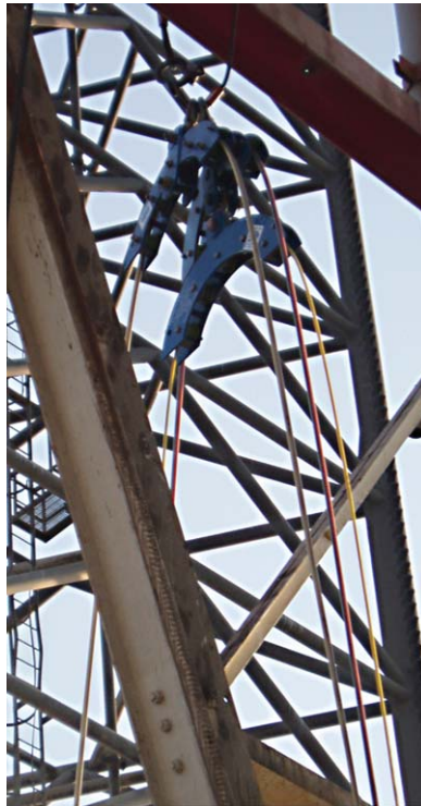
Figure 11.24 Three control lines and sheaves.
