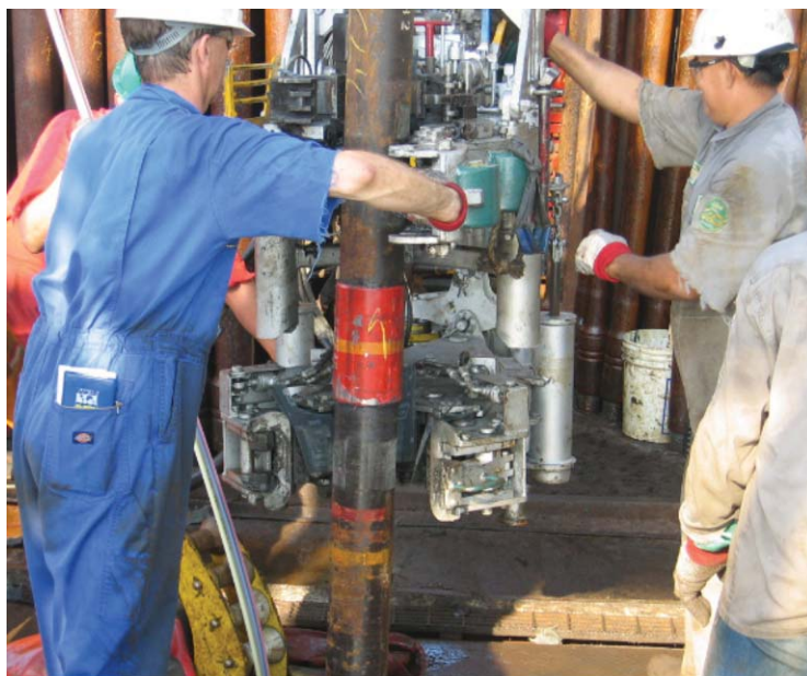
Figure 11.21 Preparing to make-up chrome tubing.
