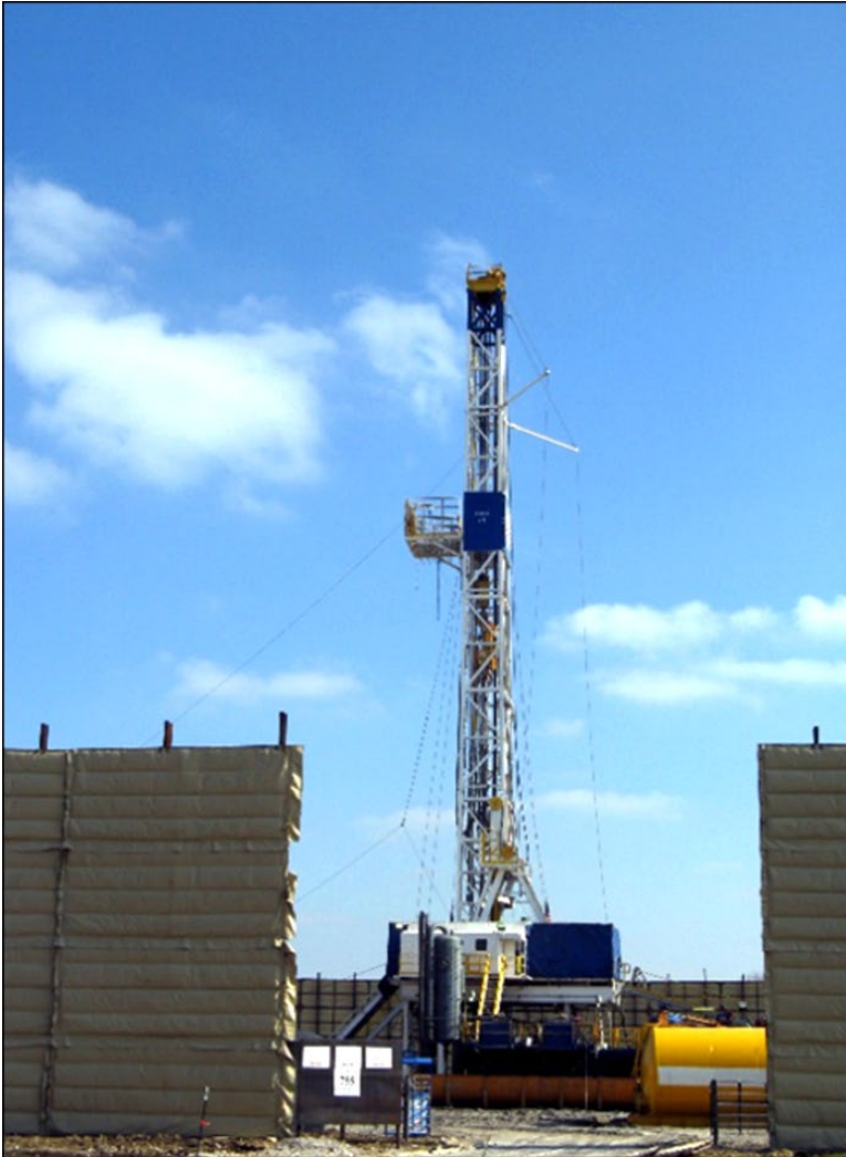
FIGURE 14.9 Drilling rig on a shale development well pad.
