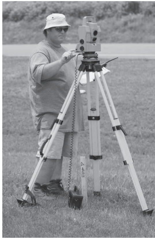
An example of an electronic distance measuring instrument used in surveying.
